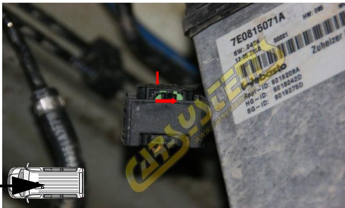
Remove plug from webasto heater. Slide green security bolt.
