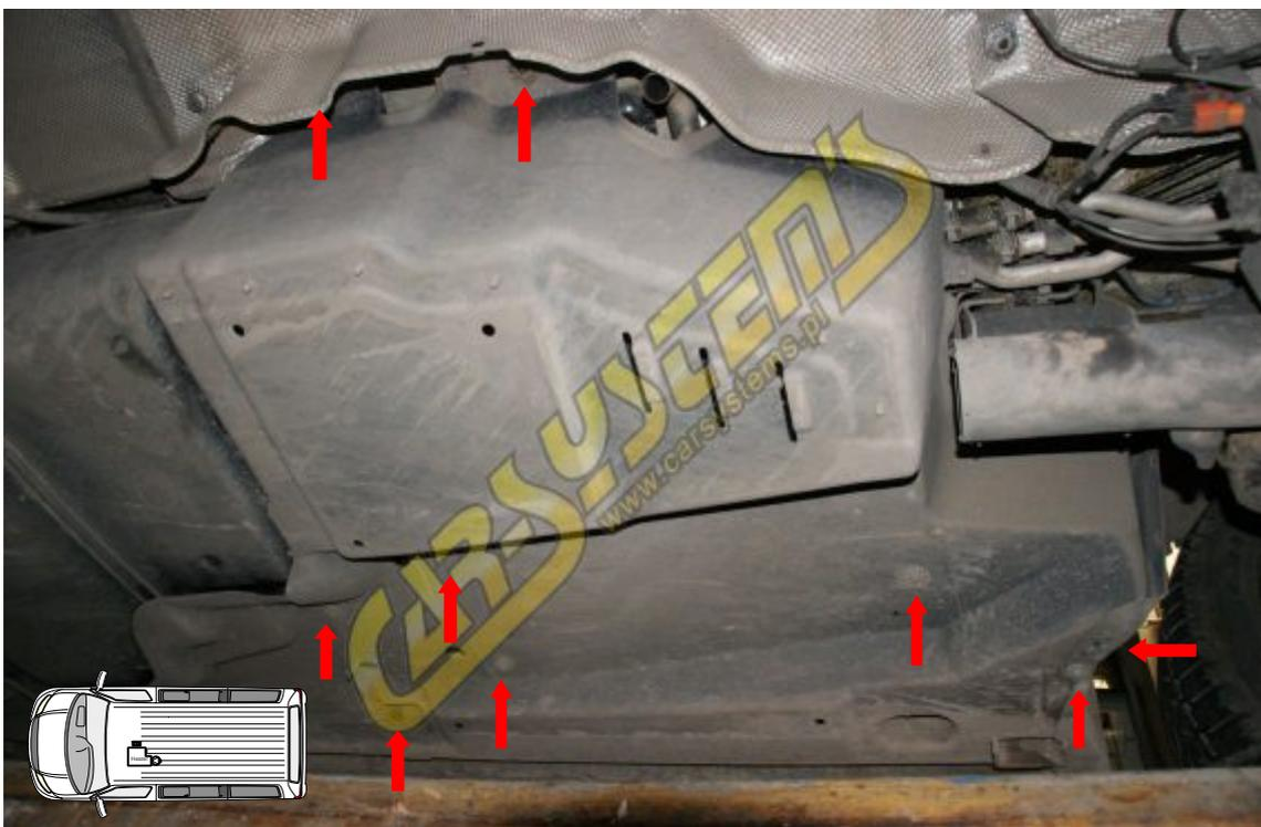
Unscrew 8mm screws, two 13mm and one T25. Remove bottom shield from car.
