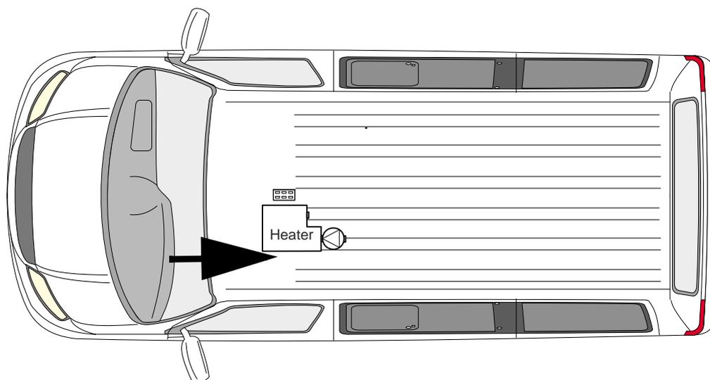
Move driver seat to the front and upper position, under the seat you will see place where telestart module should be located.
